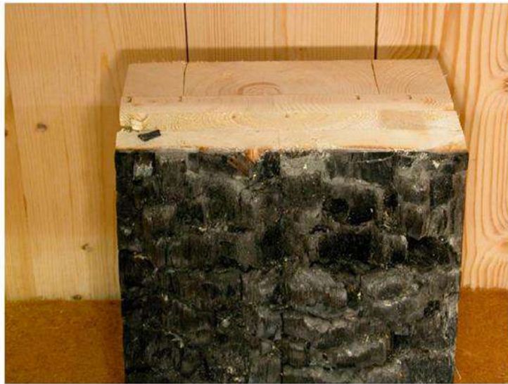
Figure 1 : Char layer and virgin wood with full strength. Source: Treteknisk Institutt
